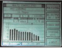
Figure 14 – 950-2150MHz – with 4-Way Splitter
